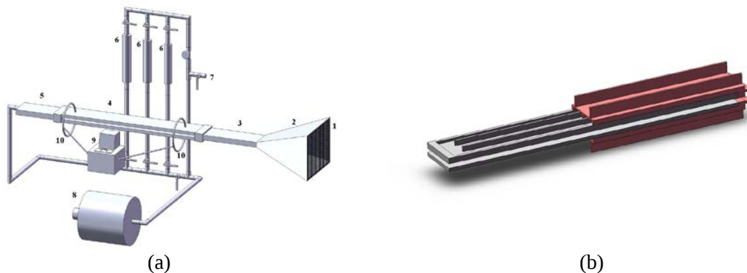
Figure 1. Schematics of the experimental setup: 1. fine mesh screen cover; 2. convergent air inlet; 3. entry-section; 4. test-section; 5. exit-section; 6. rotameters; 7. by-pass; 8. blower; 9. heat bath; 10. water circuit piping (a), test section with the duct on the wall backside (b)
