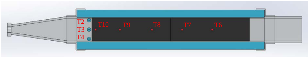
Figure 2. Temperature probes, test section.
