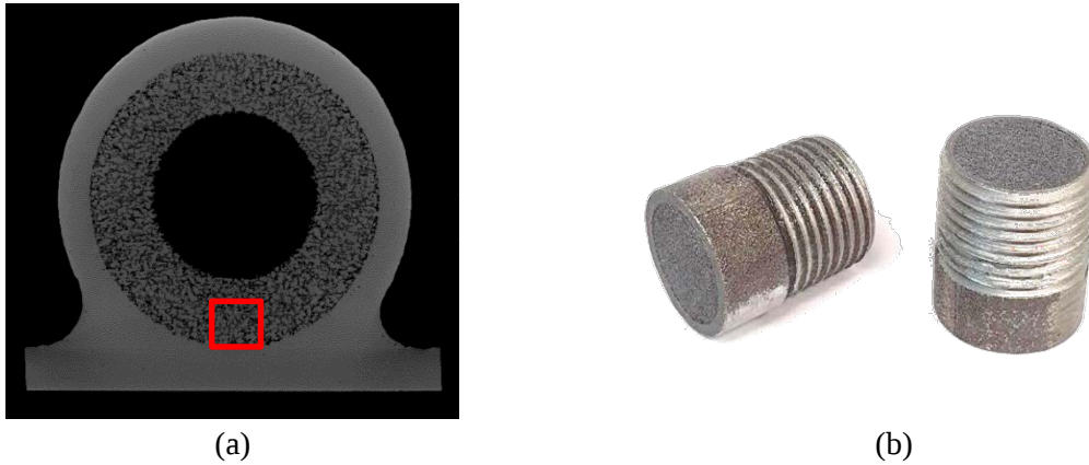
Figure 1. Tomographed heat pipe section with highlight of the wick portion used for computational analyses (a) and samples for the direct measurement permeability test (b).
